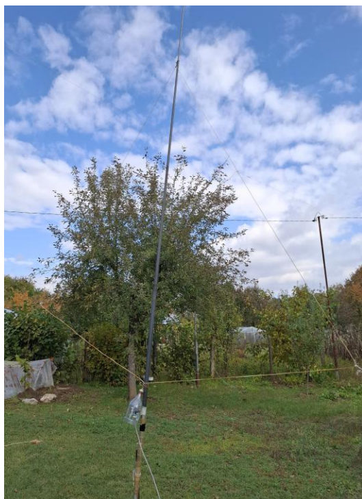
Fig. 6 Single turn triangle wire loop with 2.7 m side
