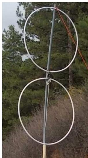
**Fig.5** Loop 5: 2 x CC loops with 0.96m diam. Loops are from PE covered 15mm diam. alum. tubes.
