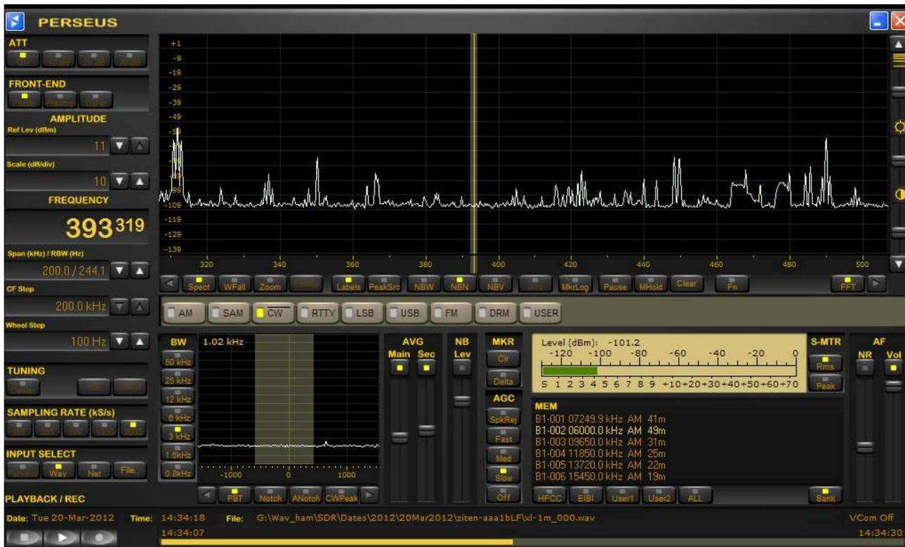
Fig.8 NDB band record with 2 CC loop antenna
