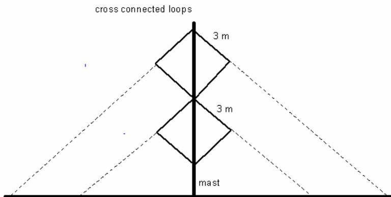
**Fig.7** High sensitivity large CC loop for LF and NDB reception, made with wire on a single mast. The dashed lines are fixing ropes.
