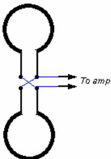
**Fig. 3** Typical parallel connection of two single turn loops in crossed coplanar (CC) scheme to reduce the equivalent inductance. The loops must lie in one plane. The equivalent loop inductance is half of the inductance of single loop and the area is twice larger.
