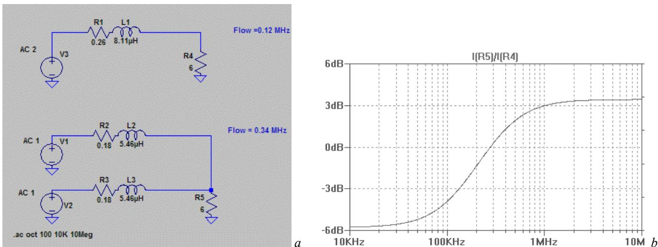
**Fig.4** Spice model of the low frequency response of a single (quad 1.41 m side) and 2 CC (two quads with 1m side) loops with equal total area and wire conductor (Cu,  $d=1\text{mm}$ ). Current ratio at 6 ohms load is shown. This load represents the input impedance of a balanced CB amplifier. Note that the induced voltage  $V3$  is twice the voltage  $V1$  or  $V2$ , since its area is two time larger than the area of each CC loop.
