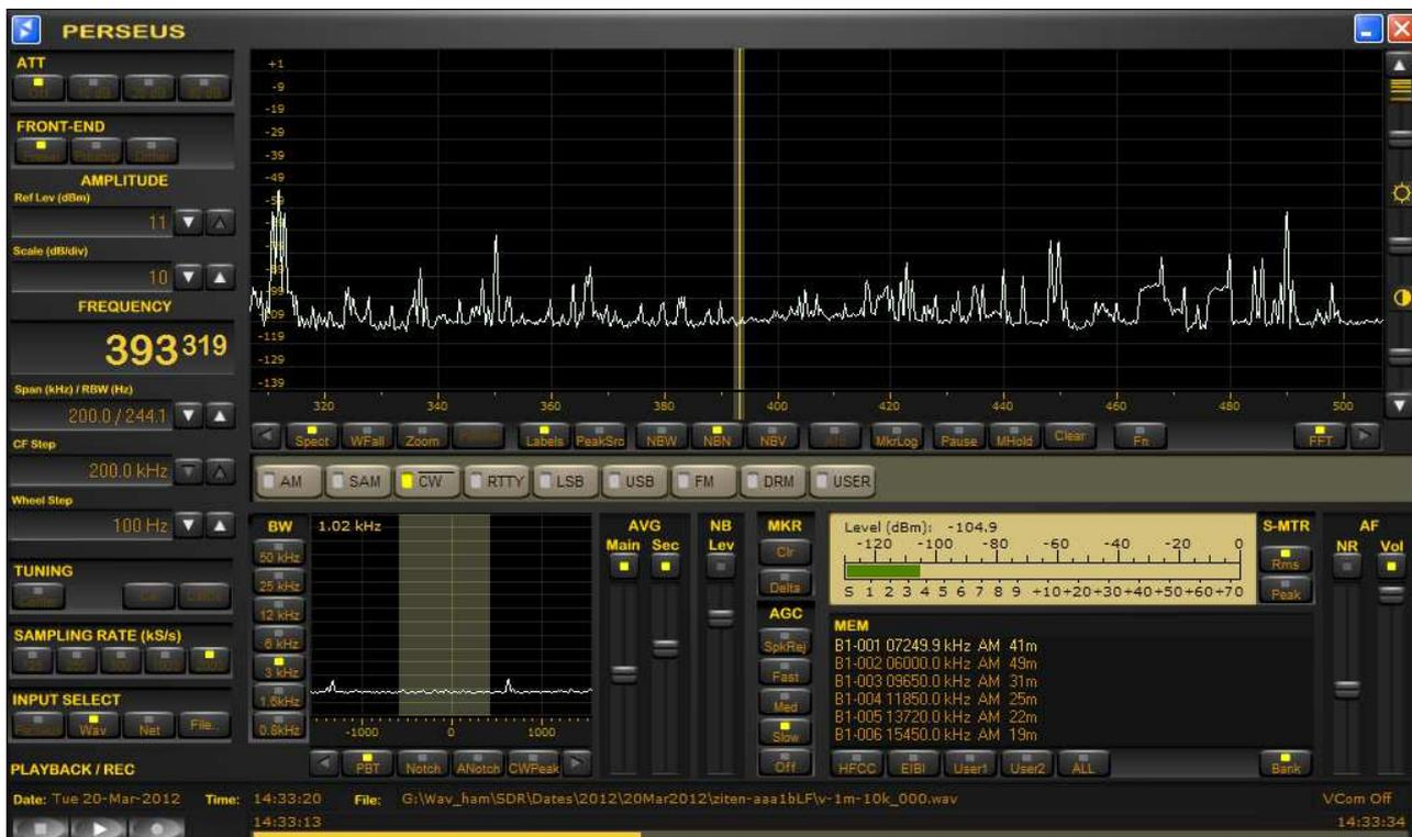
Fig.9 NDB band record with small vertical dipole antenna
